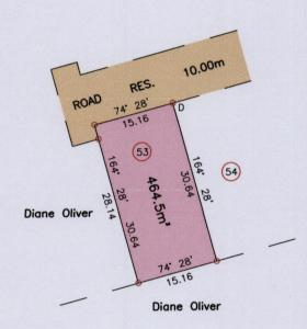
Ir.pt.=D:-N:1170058m E:691020m UTM 20, NAP Datum ±7m GPS (Hand Held) SCALE 1/750
