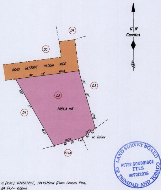
Coordinates of G (Ir.fd.): 0745672mE, 1241976mN (From General Plan) U.T.M. 20 WGS 84 (+/- 4.00m) G.P.S Direct Observation using hand-held receiver
