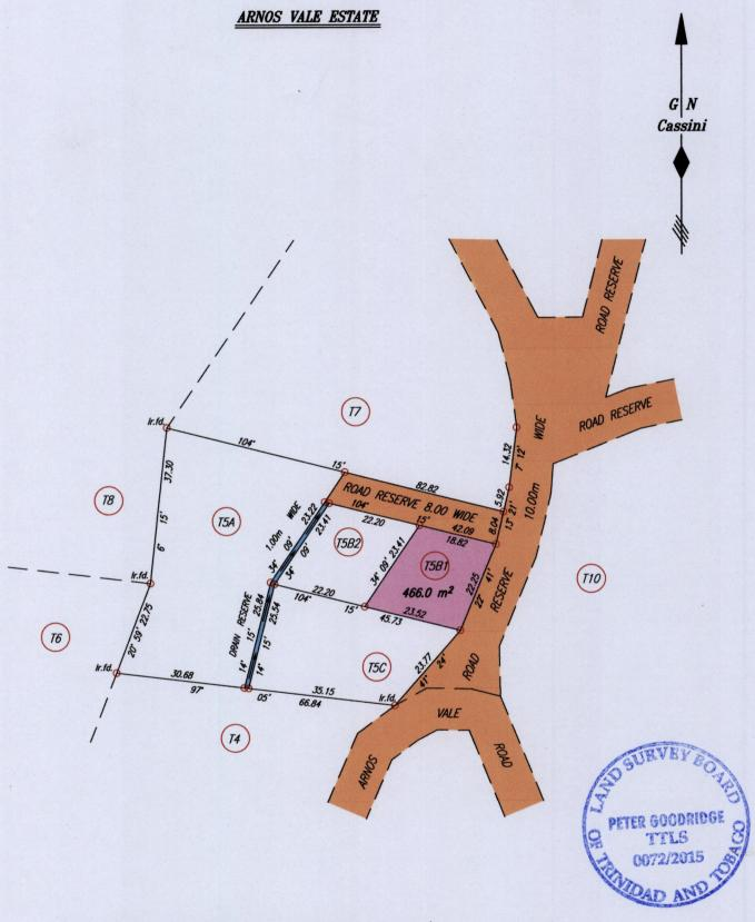
Coordinates of G (Ir.fd.) 0745672mE, 1241976mN (from General Plan) U.T.M. 20WGS 84 (+/- 4.00m) G.P.S. Direct Observation using hand held receiver
