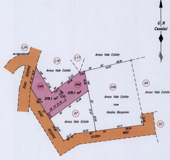
Coordinates of G (Ir.fd.): 0745672mE, 1241976mN (From General Plan) U.T.M. 20 WGS 84 (+/- 4.00m) G.P.S Direct Observation using hand-held receiver
