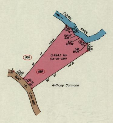
$Z = \begin{matrix} N & 1152556m \\ E & 677766m \end{matrix}$  U.T.M. 20, WGS 84 (+/-7m) Coordinates obtained from Hand held GPS.
