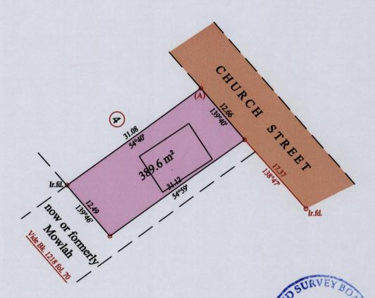
At Station (A) E 0665723 N 1132901 Reading taken with Handheld G.P.S. U.T.M. Zone 20 Naparima + 5 m.
