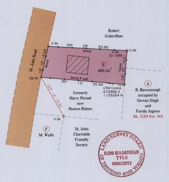
Note - UTM (Nap Zone 20) Coordinates obtained from hand held GPS receiver + 5.00m
