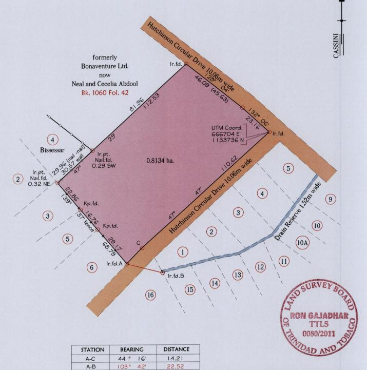
Note - UTM (Nap Zone) Coordinates obtained from hand held GPS receiver + 5.00m
