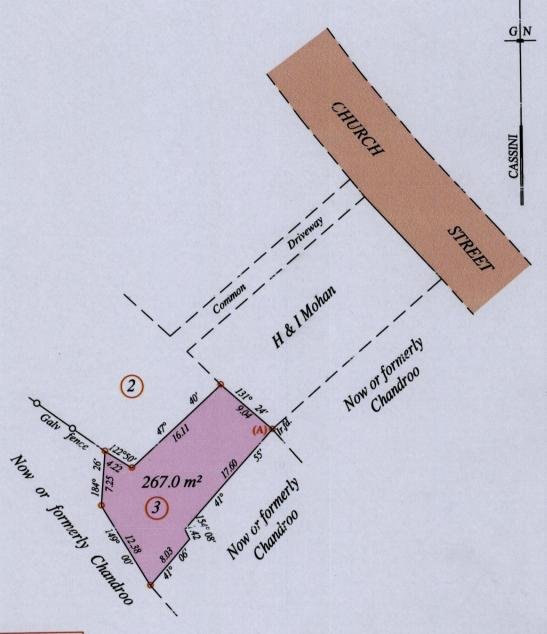
At Station (A) E 0665735 N 1132844 Reading taken with Handheld G.P.S. Garmin 76S U.T.M. Zone 20
