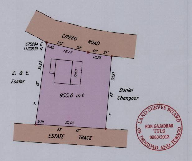
Note - UTM (NAP) Coordinates obtained from hand held GPS receiver + 5.00m
