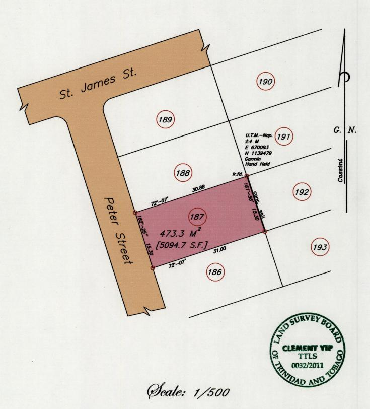
O Denotes Ir. pt. unless stated otherwise. Bearings are based on Solar Observations. Distances are in Metres. PLAN of a parcel of land coloured pink in the Ward of Naparima Containing Four Hundred and seventy three point three sq. Metres. Surveyed by me with due authority, in Dec. 2011 For Simon Baldeo
