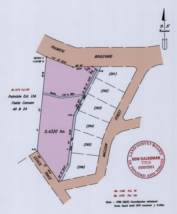
O Denotes Iron put, except otherwise stated. Note: Bearings are Cassin Grid based on Solar Obs. SCALE:- 1:1000 Distances are in metres
