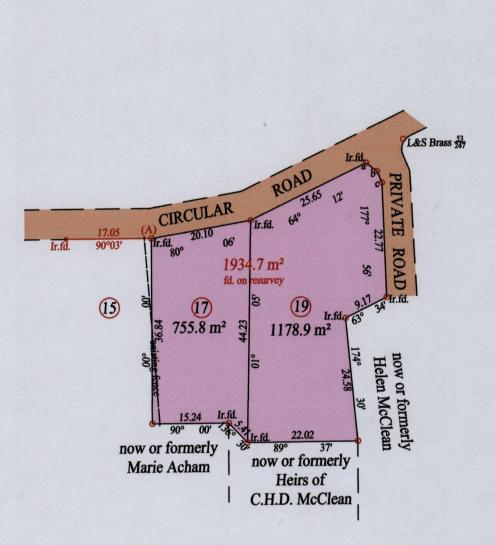
TTLS 0067/2011 At Station (A) E 0668709 N 1137080 Reading taken with Handheld G.P.S. U.T.M. Zone 20 Naparima + 5 m.
