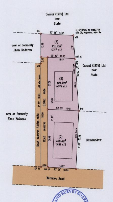
o Denotes Iron Put unless otherwise stated Bearings are Cassini Grid based on Solar Obs. Scale 1:500 Distances are in metres
