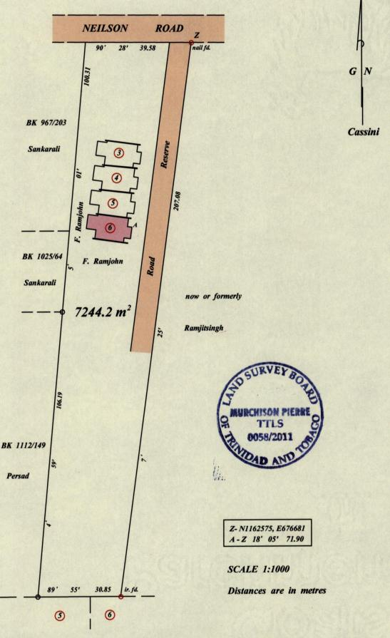
Coordinates taken on hand held Magellan GPS Receiver +/\_ 5 metres point Z Bearings are Cassini Grid based on Solar Observations
