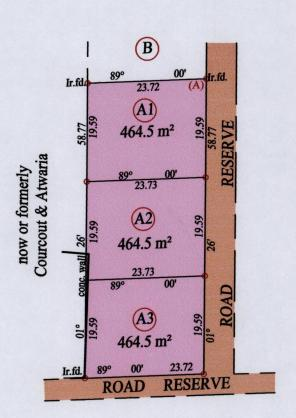
At Station (A) E 0679950 N 1169873 Reading taken with Handheld G.P.S. U.T.M. Zone 20 Naparima + 5 m.
