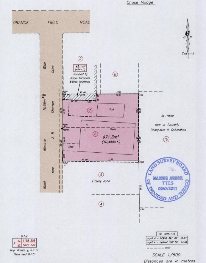
O Denotes Nail Put unless otherwise stated Bearings are Cassini Grid based on Solar Observations PLAN of a Parcel of land coloured pink in the Ward of Chaguanas Containing nine seven one point three square metres Surveyed by me, with due authority, in September 2011 for Javan Charran In accordance with Regulation 25 (1) of the Land Surveyors' Regulations 1998 LAND AND MARINE AFFAIRS I certify that this plan is correct.
