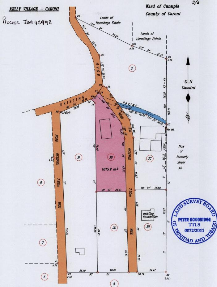
Coordinates of A (Ir. fd.): 0679716mE, 1170346mN UTM 20 WGS 84 (+/- 5m) G.P.S. Direct Observation using handheld GPS
