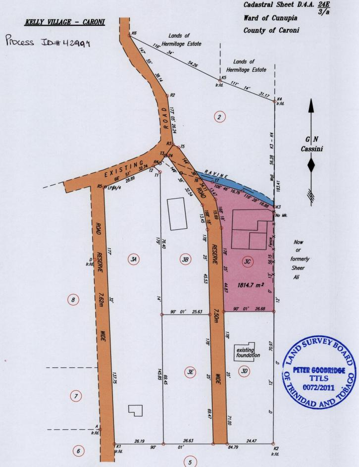
Coordinates of A (Ir. fd.): 0679716mE, 1170346mN UTM 20 WGS 84 (+/- 5m) G.P.S. Direct Observation using handheld GPS
