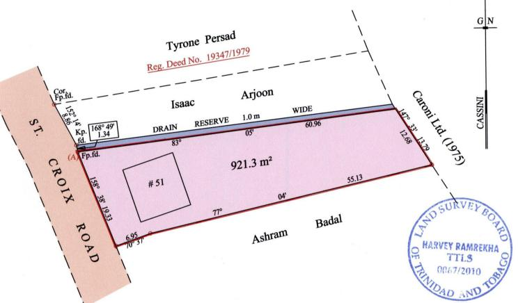
Statiom (A) E 0678477 N 1134997 Reading taken with Handheld G.P.S. U.T.M. Zone 20 Naparima + 5 m.
