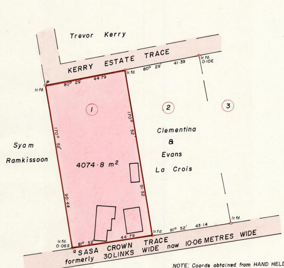
NOTE: Coords obtained from HAND HELD RECEIVER. To be used for Parcel Identification only. DATUM WGS 84 : PROJ. U.T. M.
