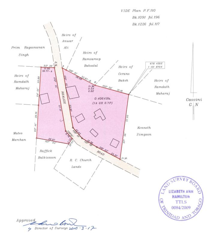
Co-ordinates are U.T.M. Zone 20 Naparima Datum +/-5m scaled from L&S 1/10000 mapping
