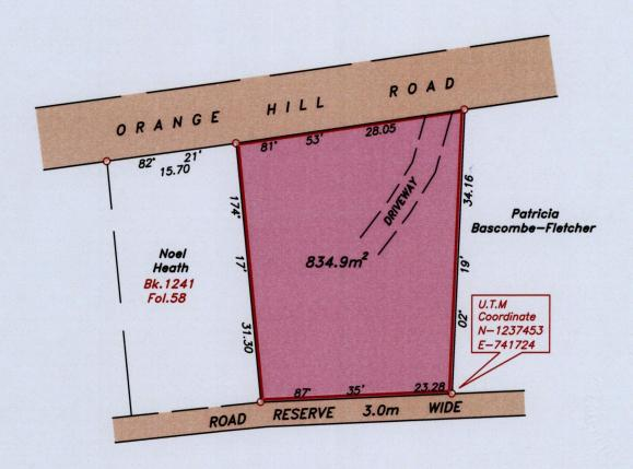
Note- UTM Zone 20 (WGS 84) Coordinates obtained from hand held GPS receiver  $\stackrel{+}{-} 6.00 \mathrm{m}$
