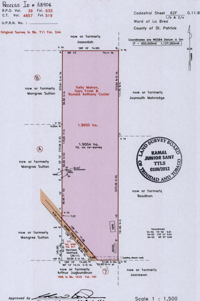
O Denotes iron put unless otherwise stated Bearings are Cassini grid based on solar observations. Coordinates are WGS84 Datum, UTM Zone 20N projection based handheld GPS. PLAN of a parcel of land coloured pink in the Ward of La Brea. Containing one point nine zero zero four hectares. Surveyed by me with due authority, on 25th August, 2012. In accordance with Regulation 25(1) of the Land Surveyors' Regulations 1998,
