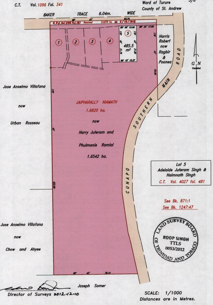
This is a true copy of a diagram of One Point Six Eight Two Zero Hectares originally transferred to JAIPHARALLY NIAMATH shewing a portion coloured pink and containing One Point Six Five Four Two Hectares being the remainder after one resumptiom and one previous transfer of other portions of the land. In accordance with Regulation 25 (1) of the Land Surveyors' Regulations 1998, I certify that this plan is correct.
