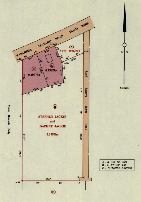
Coordinates taken on hand held Magellan GPS Receiver WGS 84 +/\_ 5 Metres point Z Bearings are Cassini Grid based on Solar Observations
