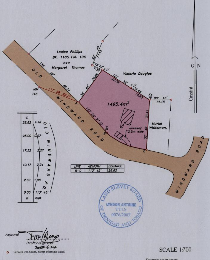
Bearings are grid based on solar observations
