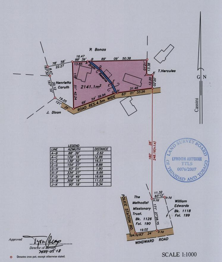
Bearings are grid based on solar observations
