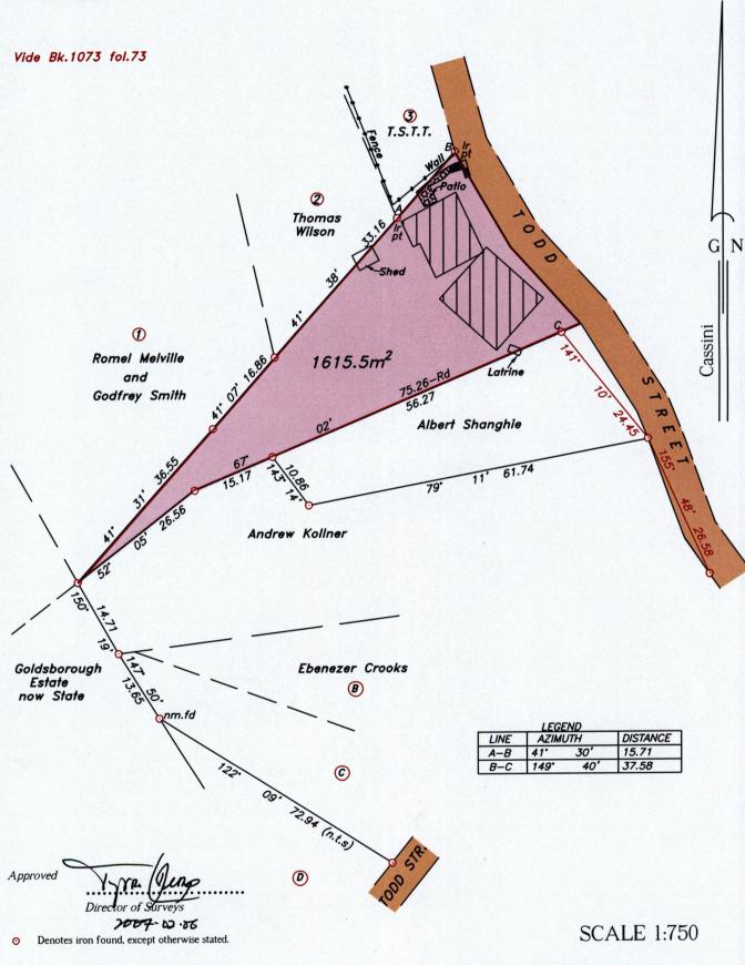
Bearings are grid based on solar observations
