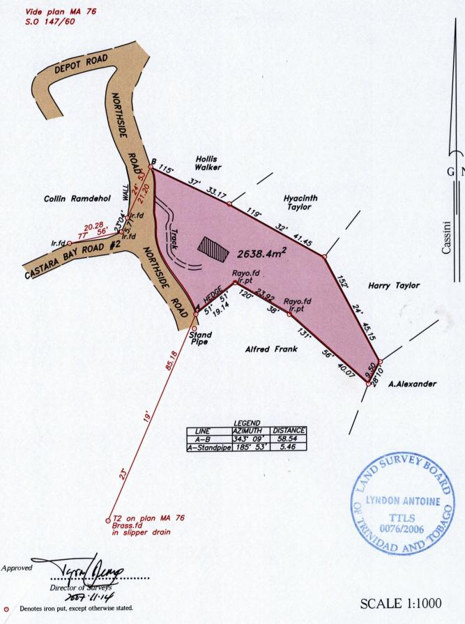
Bearings are grid based on solar observations
