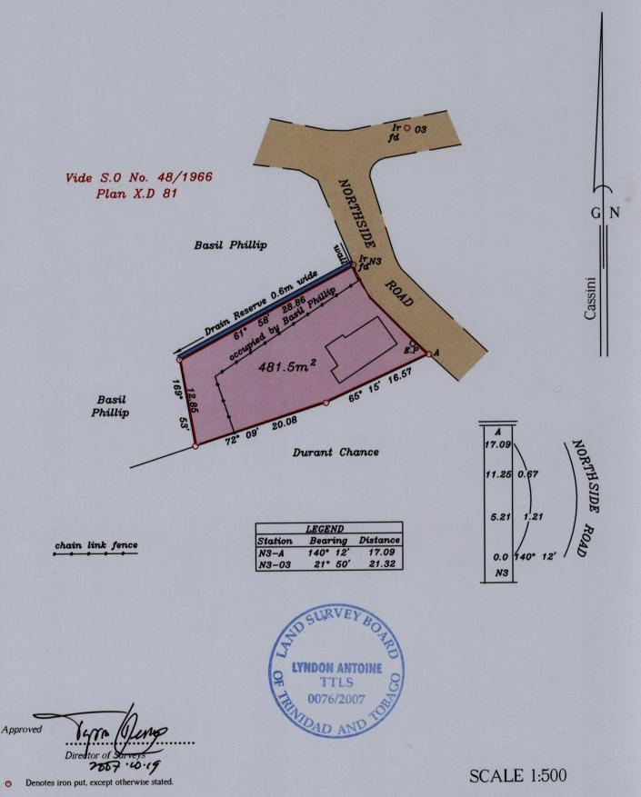
Bearings are grid based on solar observations
