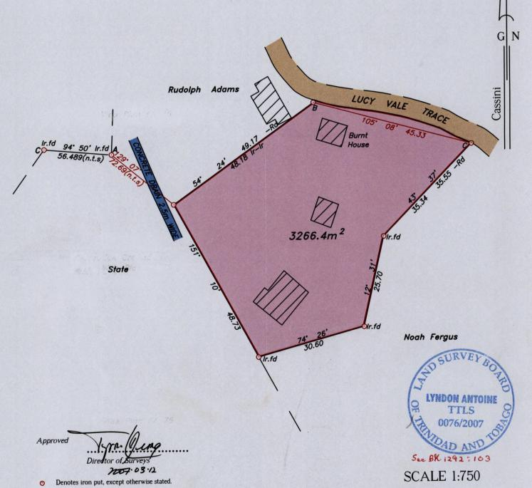
Bearings are grid based on solar observations
