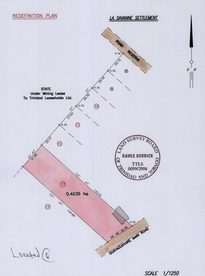
Distances are in Metres Bearings are Cassini Grid based on Solar Observations Plan of a Parcel of land coloured pink in the Ward of Guayaguayare Containing zero point four zero three five hectare Surveyed by me with due authority, in March 2006 for Eastern Emergency Response Srevices Ltd. In accordance with Regulation 25 (1) of the Land Surveyors' Regulations 1998,
