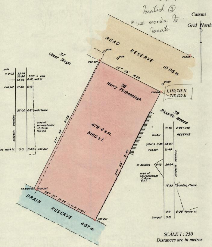
Bearings are Cassini Grid, based on solar observations. To obtain compass bearings add 14 minutes.
