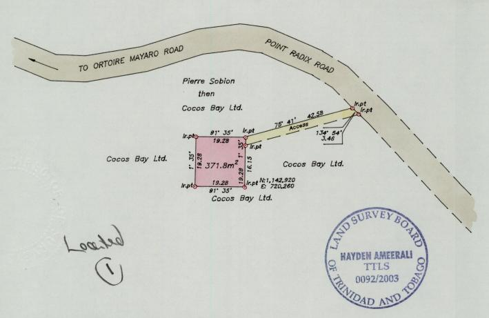
Bearings are Cassini grid based on Magnetic Needle Note: To obtain compass bearings add 18 minutes.
