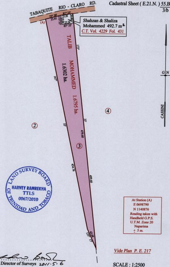
Note: Bearings are cassini grid based on solar observations Distances are in metres This is a true copy of a diagram of one point six seven nine five hectare, originally transfered to Talib Mohammed, shewing a portion coloured pink and containing one point six three zero two hectare being the remainder after one (1) previous transfer of another portion of the land. In accordance with Regulation 25 (1) of the Land Surveyors' Regulations 1998, I certify that this plan is correct.
