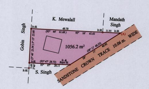
At Station (A) E 0676559 N 1142505 Reading taken with Handheld G.P.S. U.T.M. Zone 20 Naparima + 5 m.
