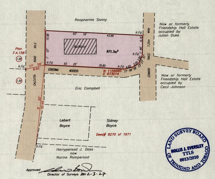
Coordinates are UTM-Nap(±5m) obtained by Handheld GPS
