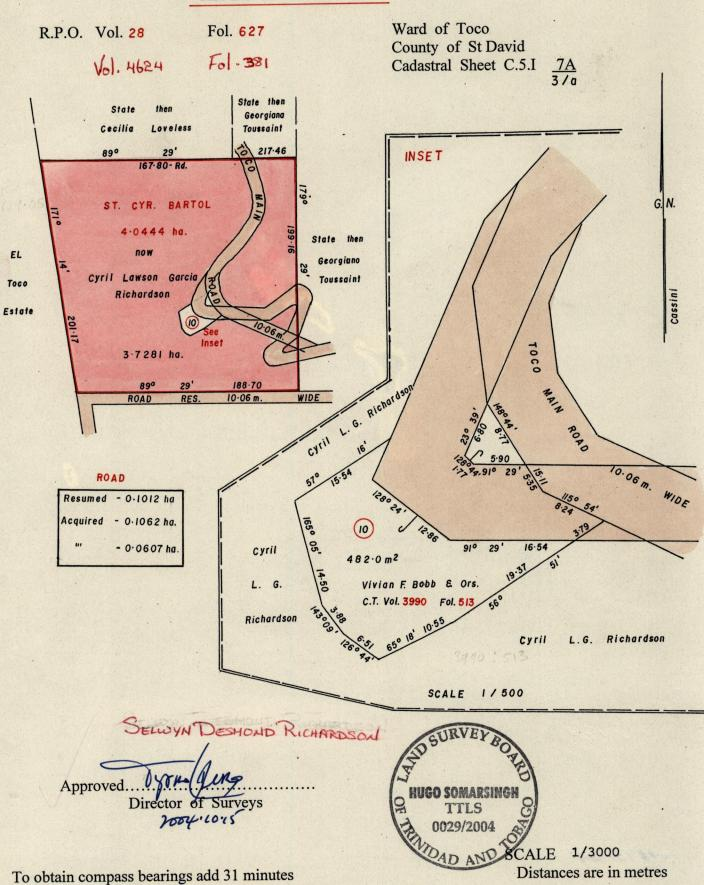
This is a true copy of a diagram of Four Point Zero Four Four Four Hectares originally granted to ST. CYR BARTOL shewing a portion coloured pink and containing Three Point Seven Two Eight One Hectares being the remainder after two acquistions, one resumptions and one previous transfer of other portion of the land. In accordance with Regulation 25 (1) of the Land Surveyors' Regulations 1998, I certify that this plan is correct.
