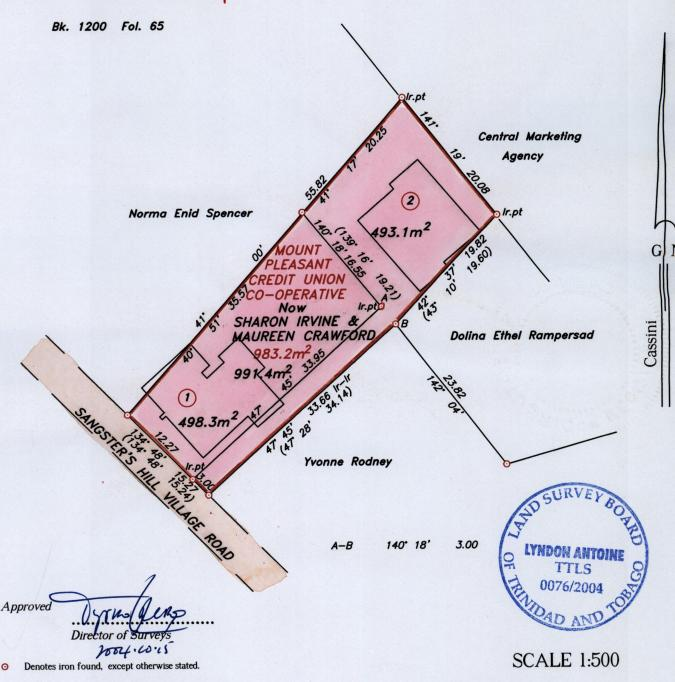
Bearings are grid based on solar observations
