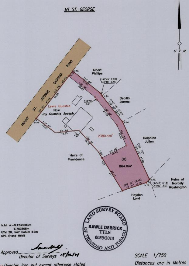
Denotes Iron put except otherwise stated Bearings are UTM Grid based on Solar Observations Plan of a Parcel of land coloured pink in the Ward of Tobago Containing eight six four point zero square metres Surveyed by me with due authority, on 2nd April 2014 Certified Correct in accordance with Regulation 25 (1) of the Land Surveyors Regulations 1998.
