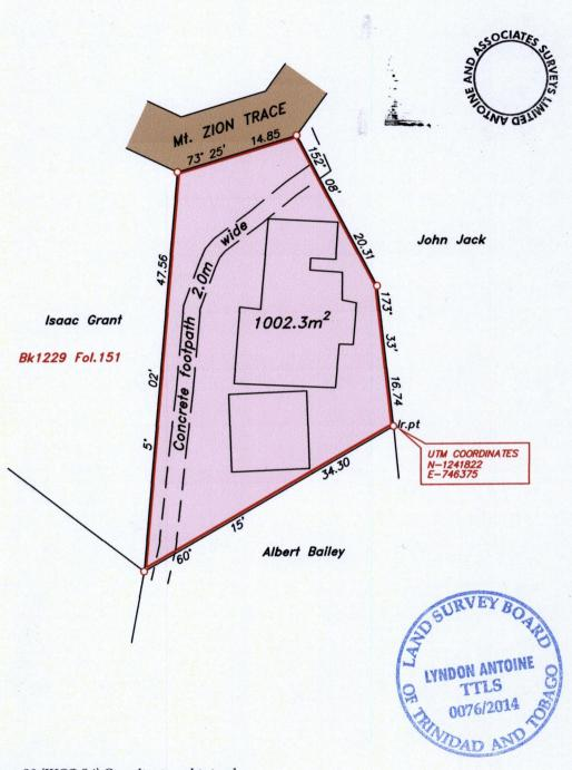
Note- UTM Zone 20 (WGS 84) Coordinates obtained from hand held GPS receiver  $^+$  5.00m
