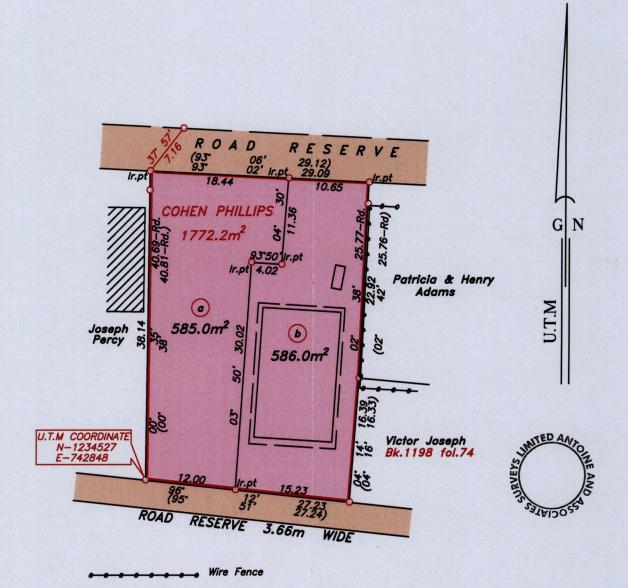
Note- UTM Zone 20 (WGS 84) Coordinates obtained from hand held GPS receiver  $^+$  5.00m
