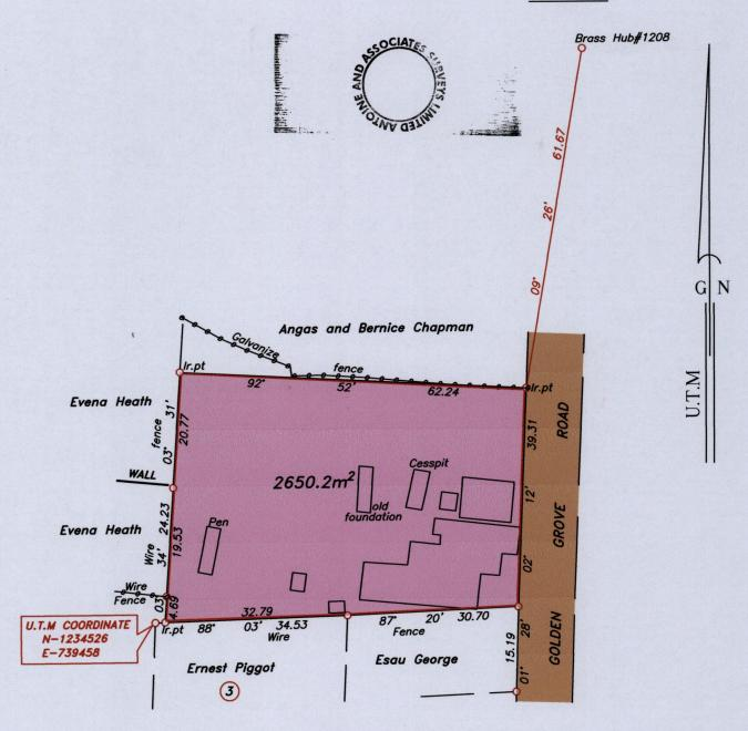
Note- UTM Zone 20 (WGS 84) Coordinates obtained from hand held GPS receiver  $\stackrel{+}{-}$  5.00m
