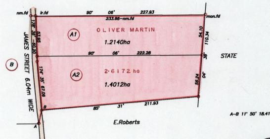
Denotes Iron put unless where otherwise stated Bearings are Cassini Grid Based on Solar Observations. Note to obtain compass bearing add/subtract minutes
