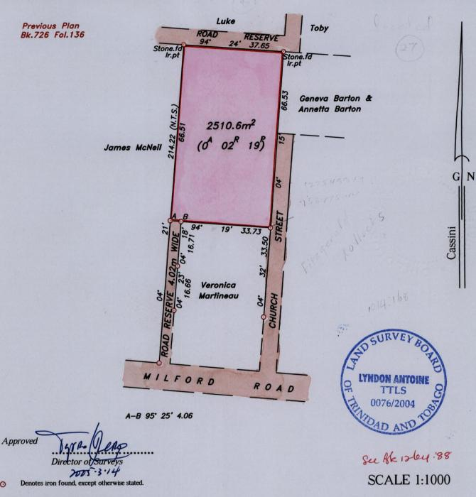
Bearings are grid based on solar observations
