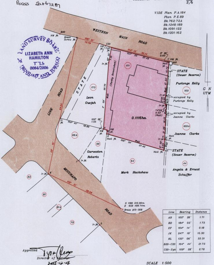
Bearings are U.T.M. Grid based on Solar Observations
