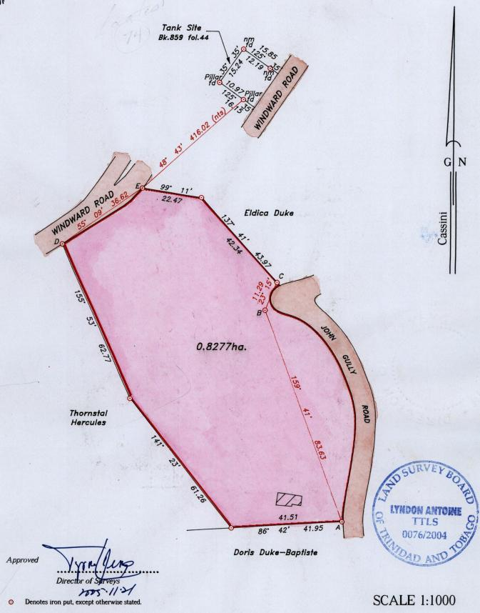
Bearings are grid based on solar observations
