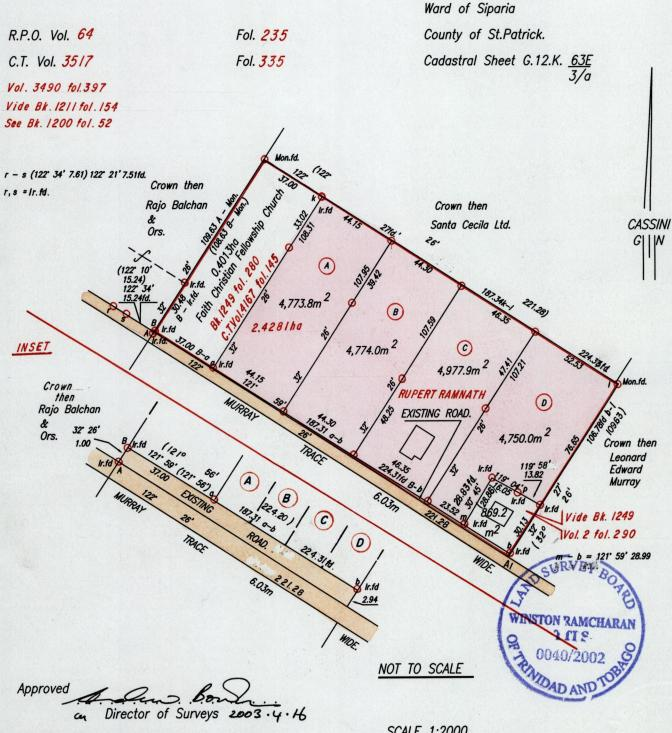
ODenotes Iron put except otherwise stated. Bearings are based on Solar Observations SCALE 1:2000 Distances are in Metres
