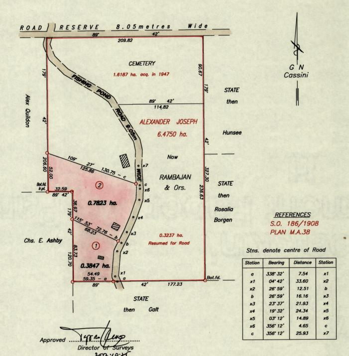
O Denotes Iron put unless otherwise stated To obtain compass bearing add 18 minutes Bearings are based on Solar observations SCALE 1:2500
